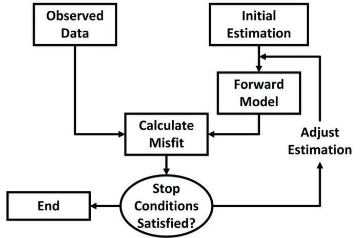
Fig. 1: In general, the target of inversion is to find a parameterized model that can fit the observed data as best
