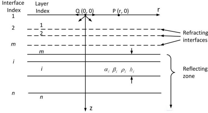
Fig. 2: The layered earth model (after [23] )
