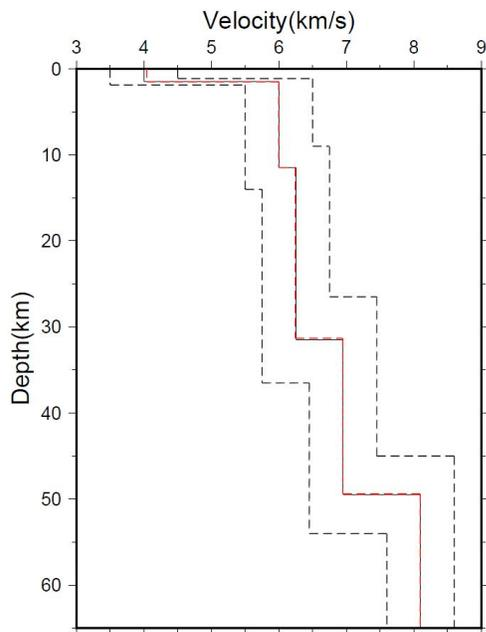
Fig. 5: Comparison between the given velocity model with the final inverted average model. Black solid line show the given model, red dashed line show the final inverted result of AR-FWA. The prescribed ranges for velocity and depth in which the model parameters are allowed to change in the inversion are shown by black dashed lines.
